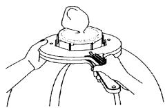
**6.** Squeeze the handles together so the prongs expand to their maximum. Lift the stretcher over and off the collar. The balloon is now loaded on the stuffing machine.
