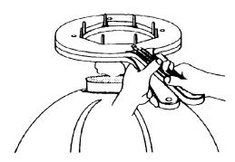
This unique balloon stretcher is designed to stretch balloons from 6" through 18". It is especially useful in mounting the smaller balloons on the rose stuffer attachment.
