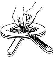
2. Simply squeeze the handles together and the prongs will stretching the balloon to fit over the machine collar.
