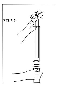
Stretch the mouth of an appropriate sized balloon over the rim of the upper tube while it is in the raised position. (See Figure 3.3)
