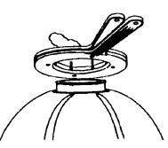
4. When the opening of the stretcher is centered over the collar lower the stretcher until the mouth of the balloon is lower than the bottom of the collar ring.
