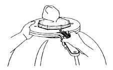
5. Releasing the pressure on the handles of the stretcher will allow the balloon to fit closely to the collar. Make sure the mouth of the balloon is below the bottom of the tabs on the collar. With a downward motion push the stretcher until the balloon releases from the prongs of the stretcher. This unique balloon stretcher is designed to stretch balloon from 6" through 18". It is especially useful in mounting the smaller balloons on the rose stuffer attachment.
