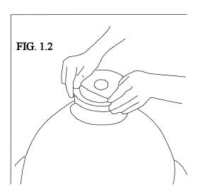
Set the inflator motor on the flat desk or table surface. The motor should have screened port facing up which is the suction side of the inflator. The end which blows is used to operate the rose stuffer, which is explained later in this manual. Plug the cord into an electrical outlet. Set the foot pedal in a convenient place on the floor.
